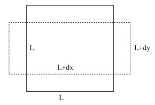
(a) Derive an expression for the Poisson ratio  $\nu \equiv -dy/dx$  in terms of the constants  $C_{ij}$ .
