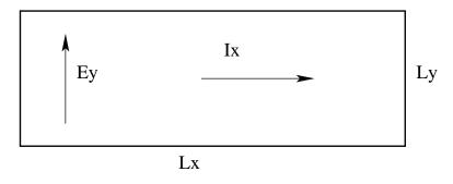
(a) Define the effective conductivity  $\sigma_{eff} \equiv j_x/E_x$  and express  $\sigma_{eff}$  in terms of the elements of the magnetoconductivity tensor  $\sigma$ .
