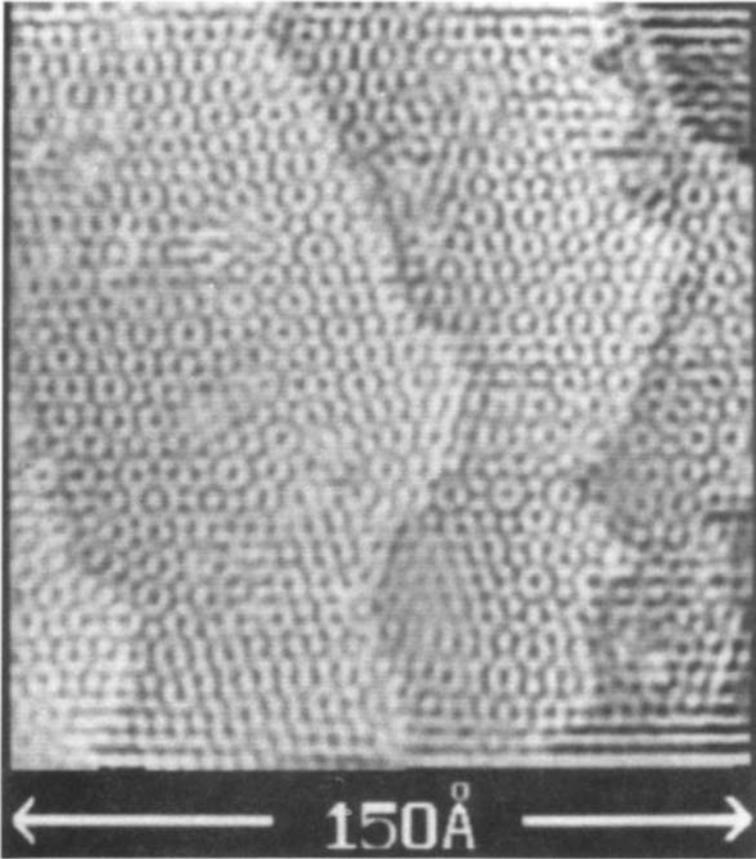
Figure 9 STM image of the surface perpendicular to the tenfold axis of decagonal Al-Cu-Co. (Courtesy of A. R. Kortan.)
