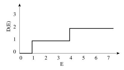
**Answer:** No state has energy less than  $E_1$ . For  $E_1 < E < E_2$ , we have D(E) constant (the motion is free in the xy plane and n = 1 along z. For  $E_2 < E < E_3$  we have both n = 1 and n = 2 z-states, each of which has a constant constribution to D(E).
