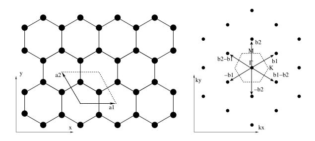
(a) Sketch and label the vectors  $\pm \mathbf{b}_1$ ,  $\pm \mathbf{b}_2$ , and  $\pm (\mathbf{b}_1 - \mathbf{b}_2)$  on the diffraction pattern.
