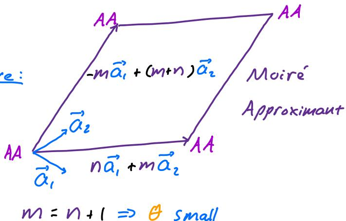
$$\text{Resonance condition: } k D_{AA} = 2\pi p \quad p \in \mathbb{Z} \quad \theta_p \approx 1/p$$
