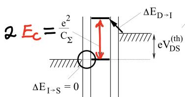
$$V_{th} = \frac{E_C C_\Sigma}{e C_D} = \frac{e}{2 C_D}$$
